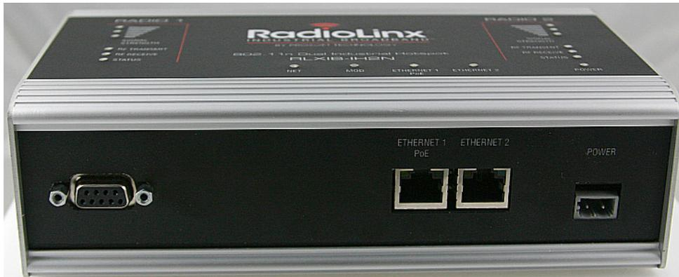
From left to right: Serial, Ethernet 1, Ethernet 2, and Power
