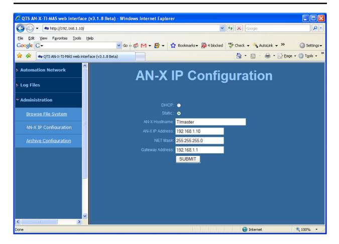
You can configure the AN-X to use DHCP or to use a static IP address.
