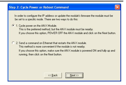
The preferred method is to cycle power on the AN-X. Select the first option on the screen and click the *Next* >> button.
