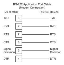
The *Use CTS Line* (page 34) parameter for the port configuration should be set to **YES** for most modem applications.
