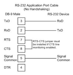
**Note:** If the port is configured with the *Use CTS* (page 34) set to **YES**, then a jumper is required between the RTS and the CTS line on the module connection.
