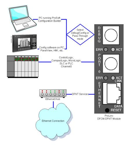
This section describes the use and configuration of the pass-through mode on the Debug/Configuration port of DFCM based modules.
