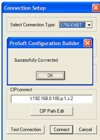
**8** Click **OK** to close the Test Connection pop-up and then click **CONNECT** to close the *Connection Set up* dialog box. The Diagnostics menu is now connected through CIPconnect.
