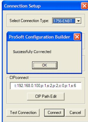
9 Click **OK** to close the Test Connection pop-up and then click **CONNECT** to close the *Connection Set up* dialog box. The Diagnostics menu is now connected through CIPconnect.
