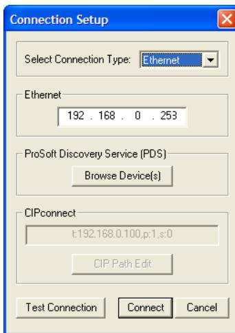
You can also use CIPconnect® to connect to the module through a 1756-ENBT card by choosing *1756-ENBT* in the **SELECT CONNECTION TYPE** list. Refer to section 3.5.1 *Using CIPconnect® to Connect to the Module* for information on how to construct a CIP path.
