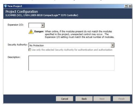
5 Select the **Expansion I/O** module number. If the modules present do not match the modules specified in the Project, unexpected control may occur. The *Expansion I/O* setting must match the actual number of modules.
