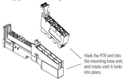
**Warning:** When you connect or disconnect the Removable Terminal Block (RTB) with the field side power applied, an electrical arc can occur. This could cause an explosion in hazardous location installations.
