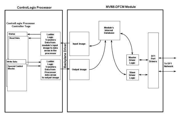
All data transferred between the module and the processor over the backplane is through the input and output images. Ladder logic must be written in the ControlLogix processor to interface the input and output image data with data defined in the Controller Tags. All data used by the module is stored in its internal database. The following illustration shows the layout of the database:
