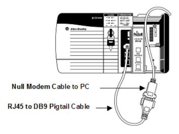
The communication port driver in *RSLinx* can occasionally prevent other applications from using the PC's COM port. If you are not able to connect to the module's configuration/debug port using *ProSoft Configuration Builder (PCB)*, *HyperTerminal* or another terminal emulator, follow these steps to disable the *RSLinx* driver.
