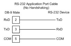
**Note:** For most null modem connections where hardware handshaking is not required, the *Use CTS Line* parameter should be set to **N** and no jumper will be required between Pins 7 (RTS) and 8 (CTS) on the connector. If the port is configured with the *Use CTS Line* set to **Y**, then a jumper is required between the RTS and the CTS lines on the port connection.
