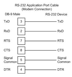
The Use CTS Line parameter for the port configuration should be set to **Y** for most modem applications.
