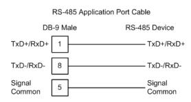
**Note:** Terminating resistors are generally not required on the RS-485 network, unless you are experiencing communication problems that can be attributed to signal echoes or reflections. In these cases, installing a 120-ohm terminating resistor between pins 1 and 8 on the module connector end of the RS-485 line may improve communication guality.
