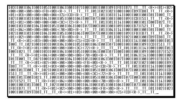
The <R+> means that the module is transitioning the communications line to a transmit state.
