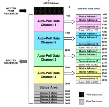
The configuration file for this example shows that when the MAX Device Address parameter is configured as 15, the module will reserve 750 words for each channel (15 devices x 50 words each) even though not all devices may be present on the network.
