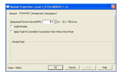
**5** Save the module. Click **OK** to dismiss the dialog box. The *Controller Organizer* window now displays the module's presence.
