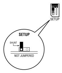
**Note:** If you are installing the module in a remote rack, you may prefer to leave the Setup pins jumpered. That way, you can update the module's firmware without requiring physical access to the module.
