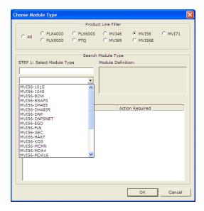
3 In the Product Line Filter area of the dialog box, select MVI56. In the Select Module Type dropdown list, select MVI56-HART, and then click OK to save your settings and return to the ProSoft Configuration Builder window.
