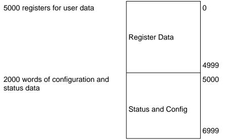
Data contained in this database is paged through the input and output images by coordination of the ControlLogix ladder logic and the MVI56-MDA4 module's program. Up to 248 words of data can be transferred from the module to the processor at a time. Up to 247 words of data can be transferred from the processor to the module. Each image has a defined structure depending on the data content and the function of the data transfer as defined below.
