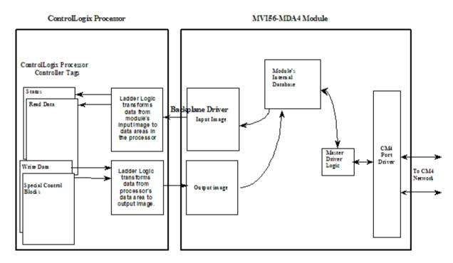
All data transferred between the module and the processor over the backplane is through the input and output images. Ladder logic must be written in the ControlLogix processor to interface the input and output image data with data defined in the Controller Tags. All data used by the module is stored in its internal database. This database is defined with addresses from 0 to 6999. The following illustration shows the layout of the database:
