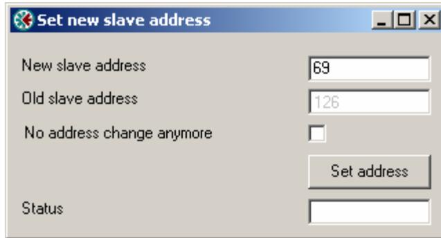
The *PROFIBUS Master Configuration* window will prevent the user from selecting a *New slave address* that is already occupied by another device; this includes detected Master stations as well. If the user selects an occupied address, a message similar to the one shown here will open.
