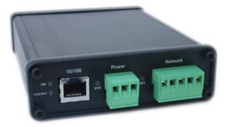
The AN-X2-SQD-MAS communications module connects to a ControlLogix PLC over Ethernet/IP and acts as a scanner on the Square D remote I/O network. It connects to CRM-220/222 adapter modules, NOT Passport I/O.
