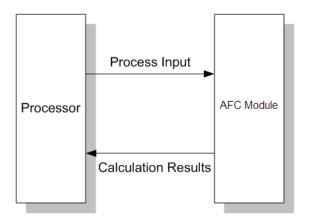
Refer to the Ladder Logic sections for instructions on how to transfer the meter process variables from the processor to the module. Ladder logic is required to move the process variables to the correct data file or controller tag in the processor. The **Meter Monitor** window (*Process Inputs* field) displays the values that are transferred from the processor.
