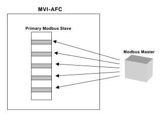
However, using the Virtual Modbus Slave optimizes the polling of data because the registers can be remapped in any order using the AFC Manager (Site Configuration window). The following illustration shows how the orifice diameter registers could be remapped to the Virtual Slave starting at address Vh00100:
