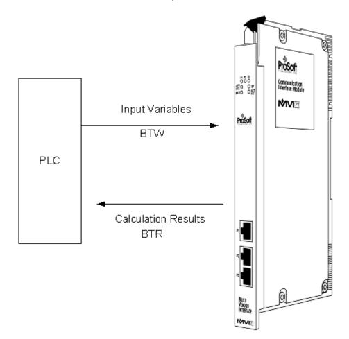
The backplane communication is also used by the processor to request some tasks from the module (including Modbus master command, set wallclock, set molar analysis data).
