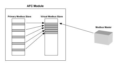
This example demonstrates the benefits of using the Virtual Slave instead of accessing the data directly from the Primary Modbus Slave. The same procedure can be used when polling data from the processor (through the backplane) because the Modbus Gateway block also requires the data to be listed in a contiguous order.
