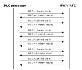
As the diagram shows, the module also periodically sends status blocks (Block Synchronization ID = -2) after every meter cycle.
