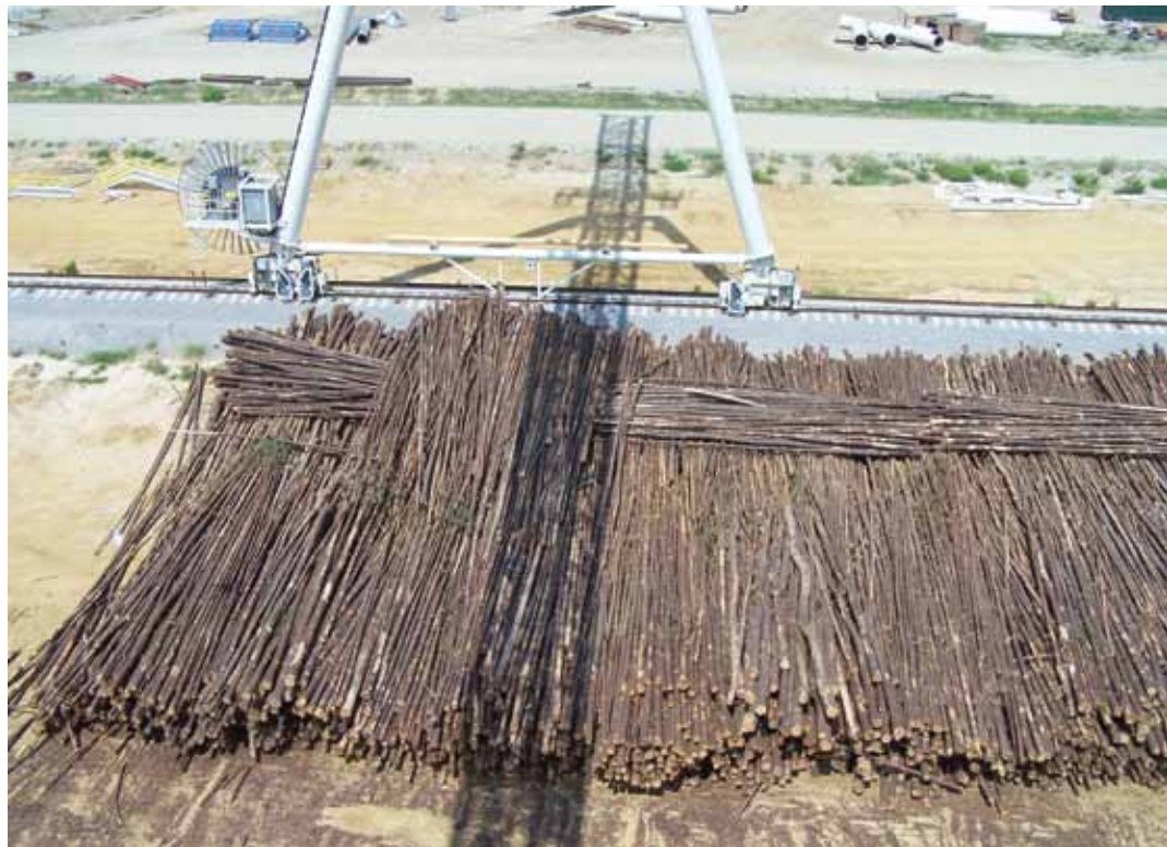
Portal Crane grapples can lift up to forty-four tons of logs in a single bite and transport them along rail runways sometimes up to a mile in length.
